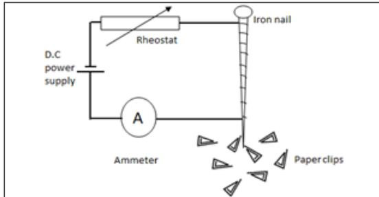
**Figure 1.** Experiment Diagram of Electromagnetism in Form 5
